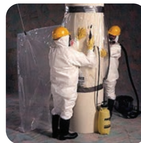
V24 Perfect for work on larger diameter vertical pipe, accommodates diameters from 10" to 24". Each bag measures 84" to 96". An offset debris area moves the weight and bulk away from the work area. One arm set, and ports per chambers, 6-mil construction.
