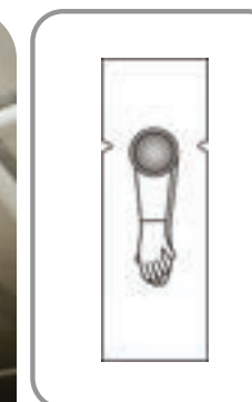
M6 The M6 is for repair and maintenance operations where the work is on small sections of insulation or gasket replacement. For pipe diameters up to 6". Each chamber measures 22"x60" with one arm set with opposing glovesleeves, 6-mil construction.
